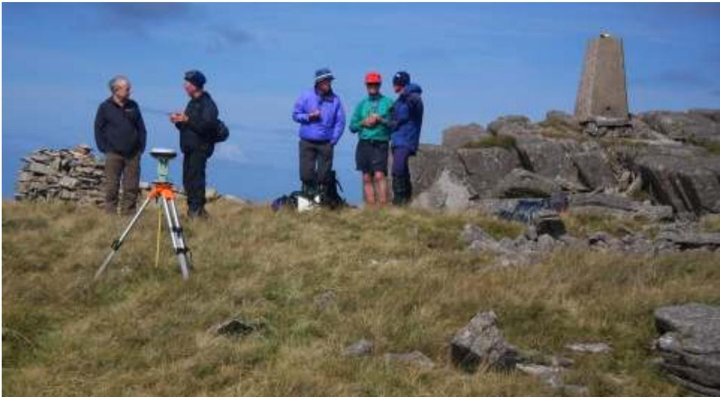
**Vertical Offset of 0.435m for Leica Viva GS15 setup on short tripod**
