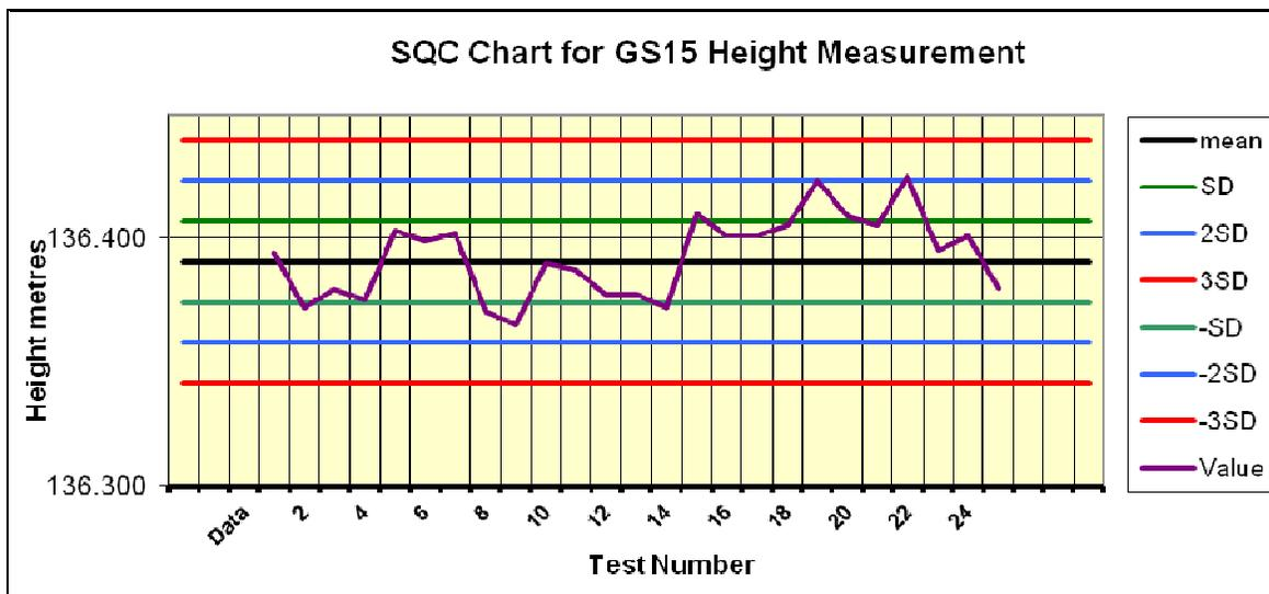
In addition, we check the instrument periodically by taking measurements on an Ordnance Survey Fundamental Bench Mark, processing the data and comparing it with the OS derived values. Height should agree to within about 0.05m. The latest two measurements are given in the table below.
