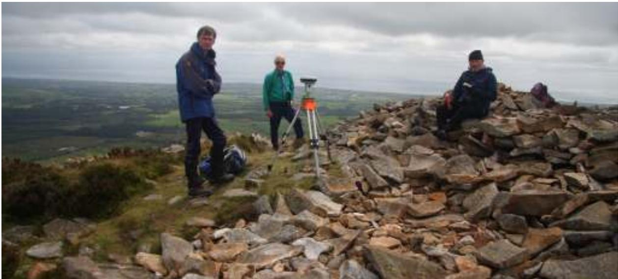
Viva GS15 setup on short tripod showing 0.594m vertical offset
