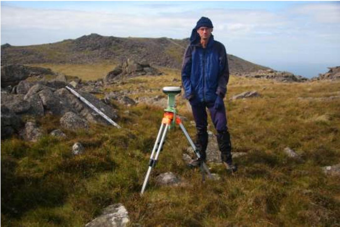
**GS15 setup position on short tripod showing 0.443m vertical offset**
