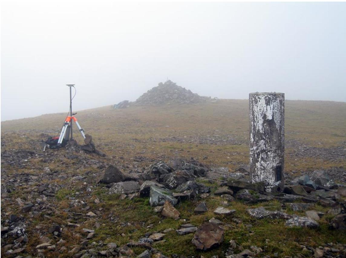
This picture shows the GPS set up on the summit position near the trig point. The base of the cairn in the background is about 0.5m lower than the summit.
