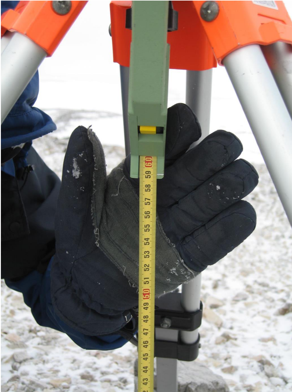
Vertical offset for Leica Viva GS15 on the summit of Carn Aosda
