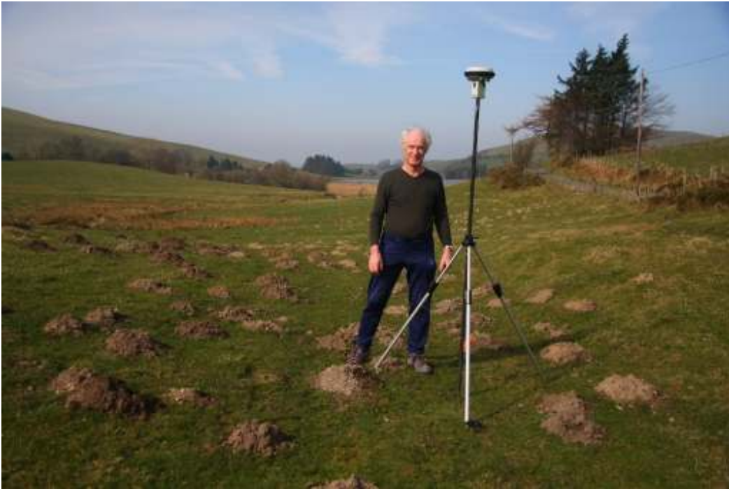
Leica GS15 set up at Bwlch – mole hills are not natural ground!!
