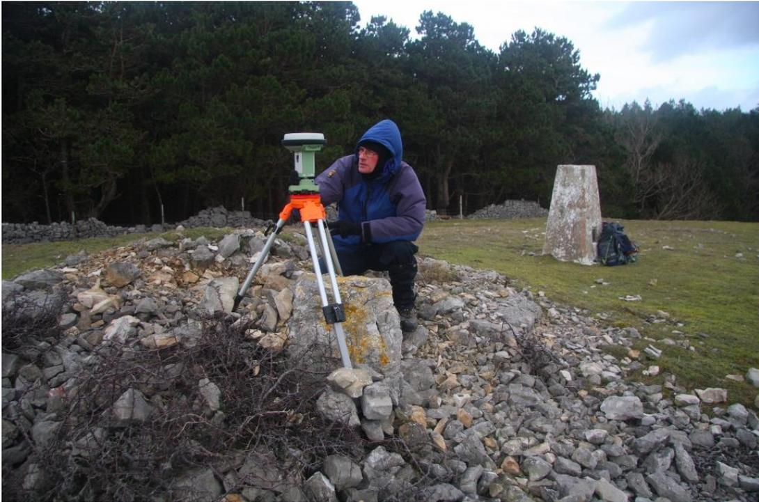
**Photograph of tape reading at summit set-up position**
