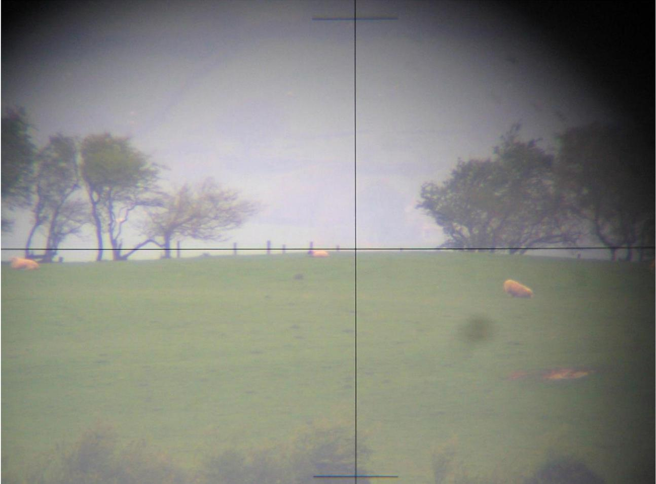
The level was set up a few metres from the summit position of Coed Mawr and aligned so that the horizontal line was level with the summit. The level was then focussed on the summit of Rhos Fawr to give the view seen in the above photograph. The horizontal line is shown cutting just above the summit of Rhos Fawr.
