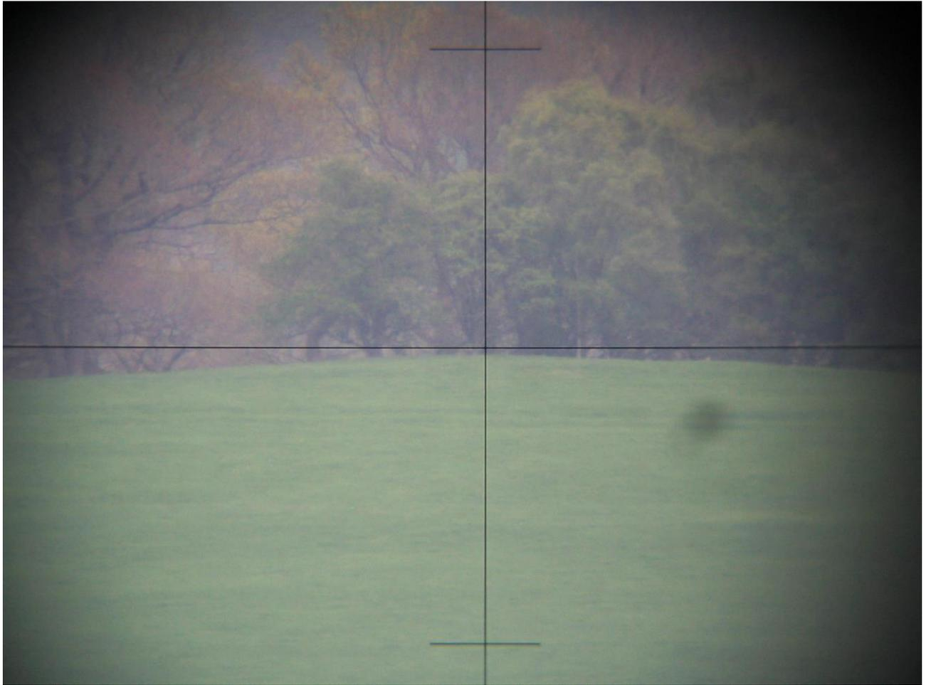
The same procedure was applied on the summit of Rhos Fawr to produce this photograph of the summit of Coed Mawr. This time the measurements from the photographs show the apparent height difference between the two summits to be 0.22m. Once again applying a value of 0.24m for earth curvature gives a result of Coed Mawr being higher than Rhos Fawr by 0.02m.
