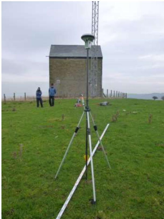
Leica Viva GS15 set up on Summit 2. Highest point is near front right corner of fence.
