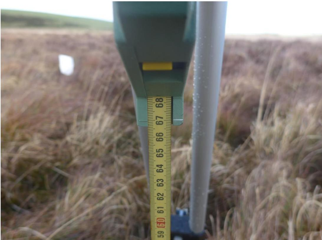
**Tape reading for Leica Viva GS15 set up on bwlch**
