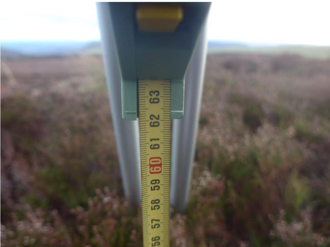
**Tape reading for Leica Viva GS15 set up on summit**
