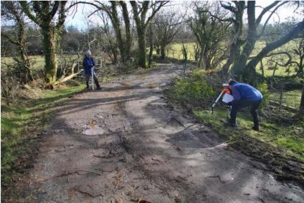
**Leica GS15 setup position with bwch in the background**
