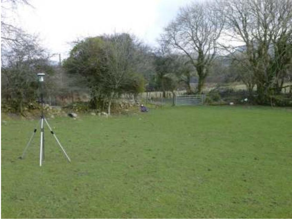
**Trimble GeoXH 6000 setup with external antenna supported on a 2.00m pole**
