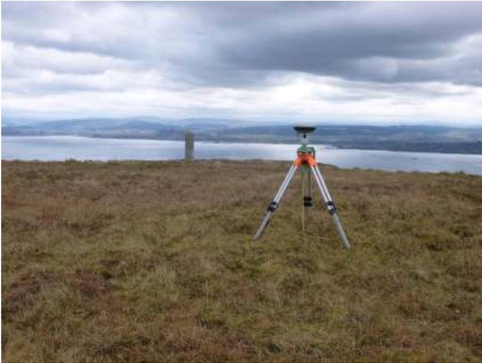
**View of GS15 set-up at summit on “short tripod”**
