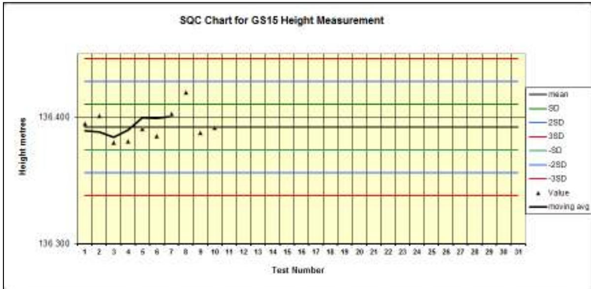
In addition, we check the instrument periodically by taking measurements on an Ordnance Survey Fundamental Bench Mark, processing the data and comparing it with the OS derived value. Heights should agree within about 0.02-0.03m.
