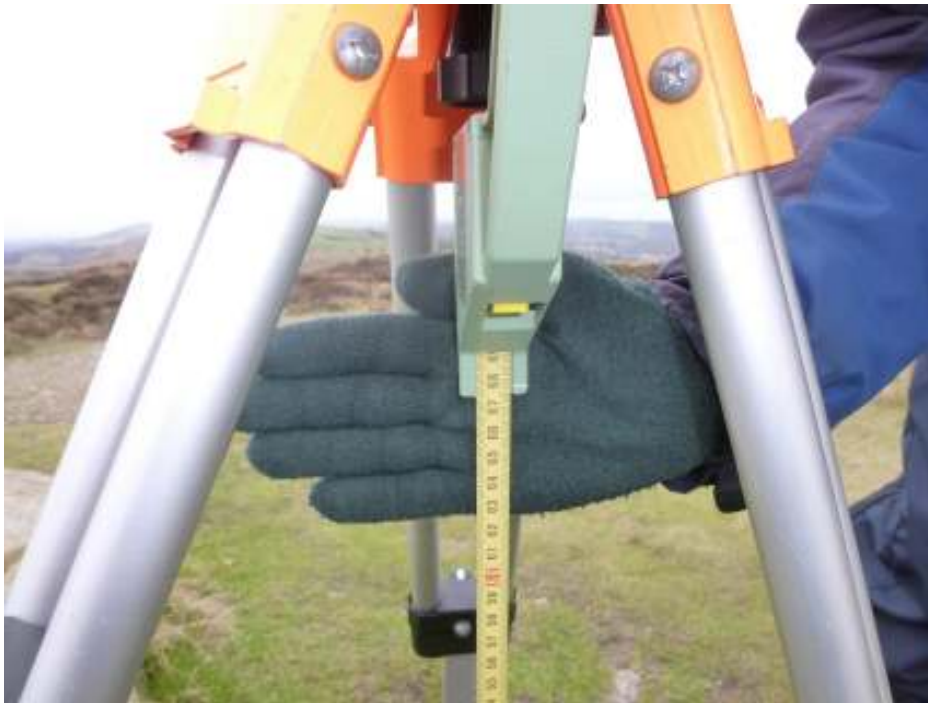
Leica GS15 Vertical offset – Tape Measurement = 0.678m
