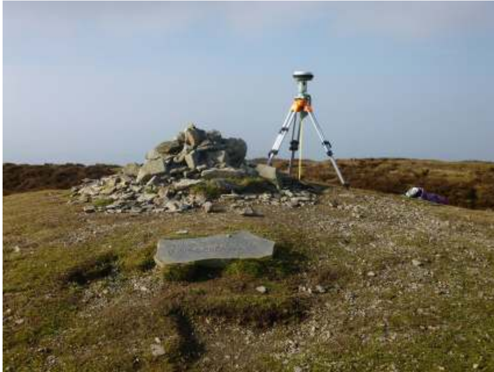
Leica GS15 (15 Feb 2015) set up at highest point on man-made mound
