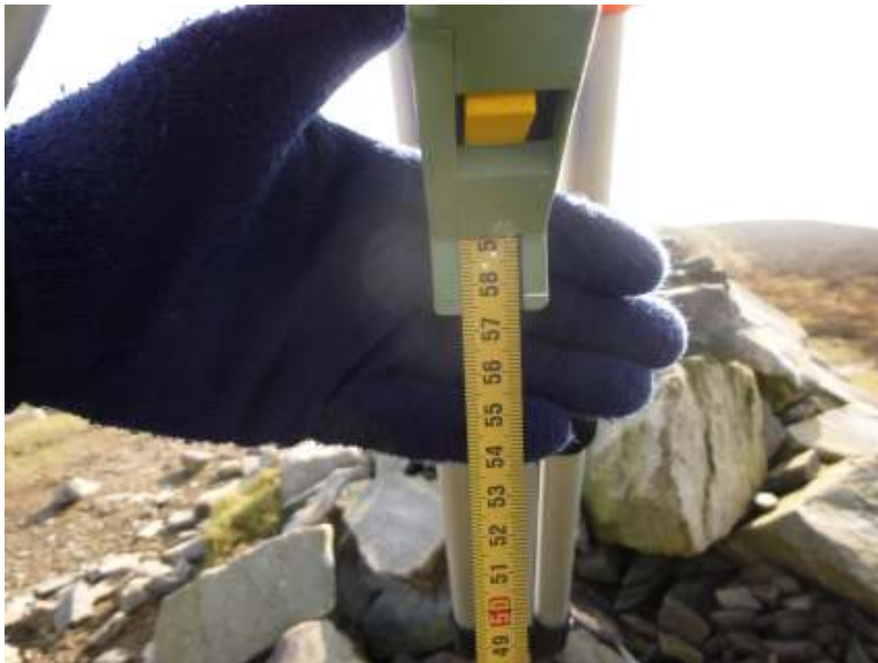
Leica GS15 Vertical offset – Tape Measurement = 0.577m
