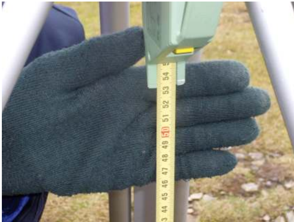
Leica GS15 Vertical offset – Tape Measurement = 0.537m
