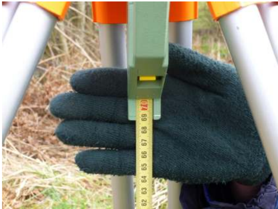
Leica GS15 Vertical offset – Tape Measurement = 0.692m
