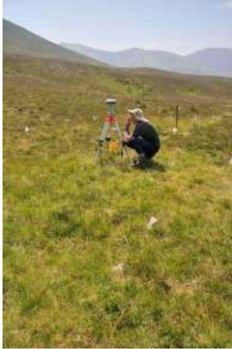
**Leica Viva GS15 set up showing vertical offset (0.738m) at the bwlch of Moel Tryfan**
