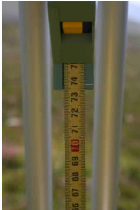
**Measuring the height of the level on small tripod on summit tor of Moel Tryfan**
