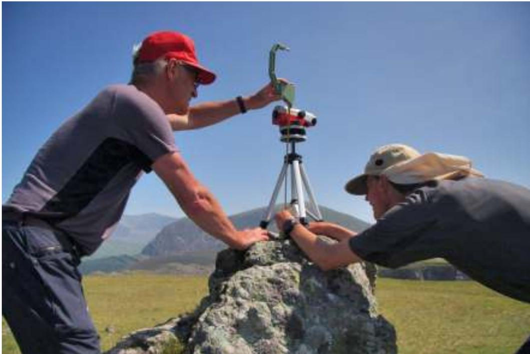
**Measuring the height difference between summit and Leica Viva GS15 set up position**
