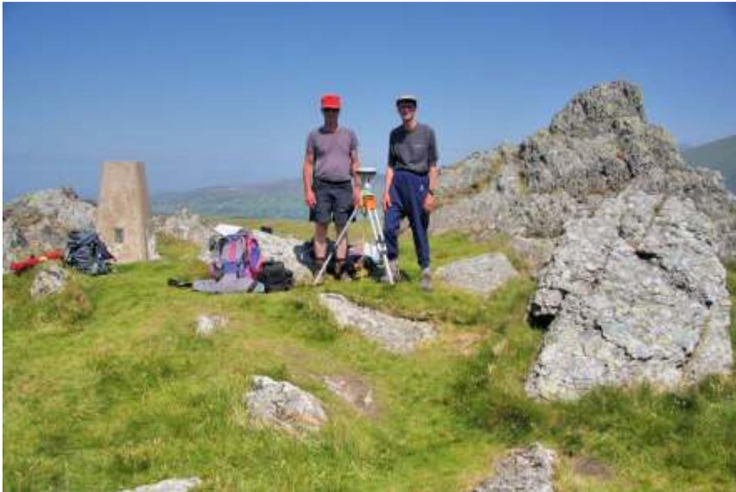
**Leica Viva GS15 set up showing vertical offset (0.645m) at the summit of Moel Tryfan**
