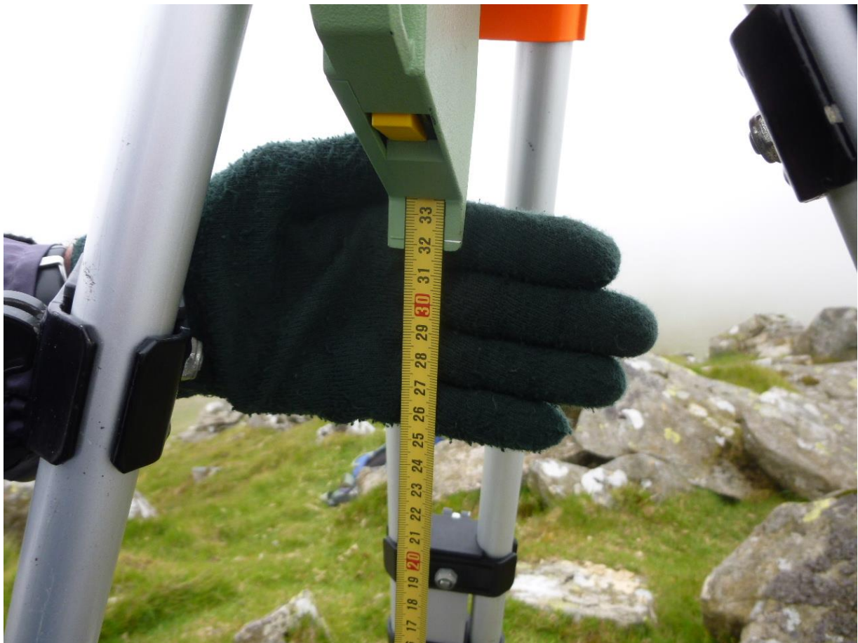
Offset for Leica Viva GS15 set-up at summit
