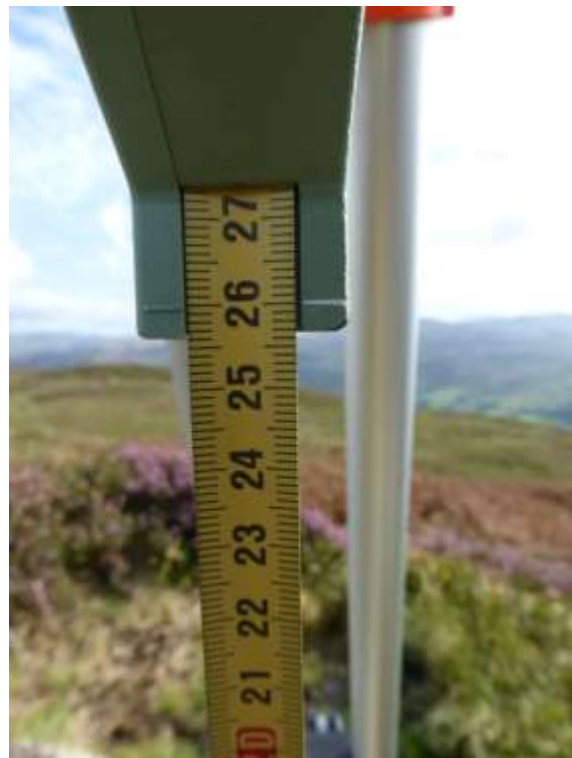
Tape reading for Leica Viva GS15 on NE Top
