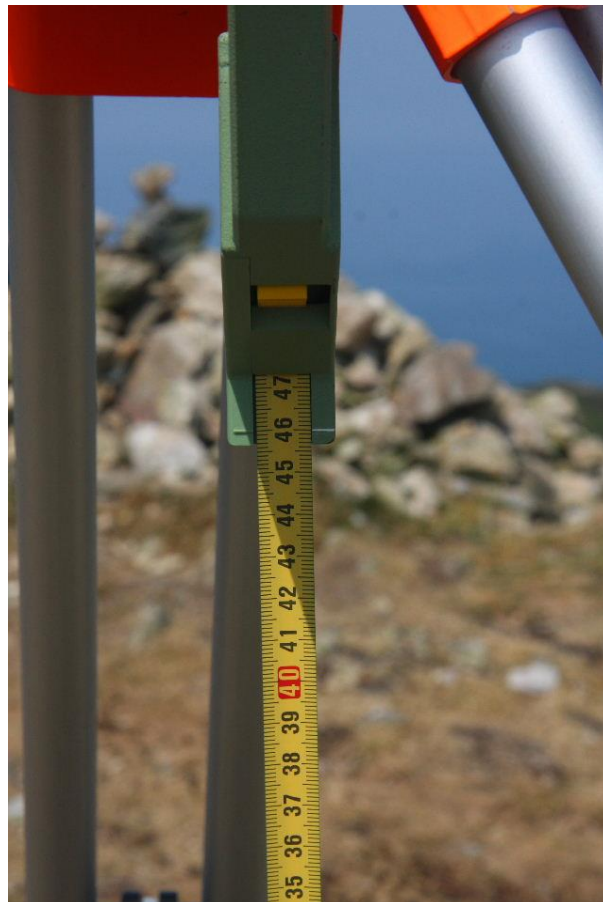
Tape reading (0.461m) for Short Tripod setup GS15 on summit
