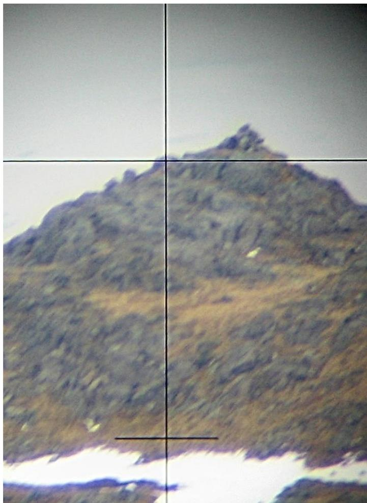
**Magnified image showing the cairn more clearly and the horizontal line passing beneath it**
