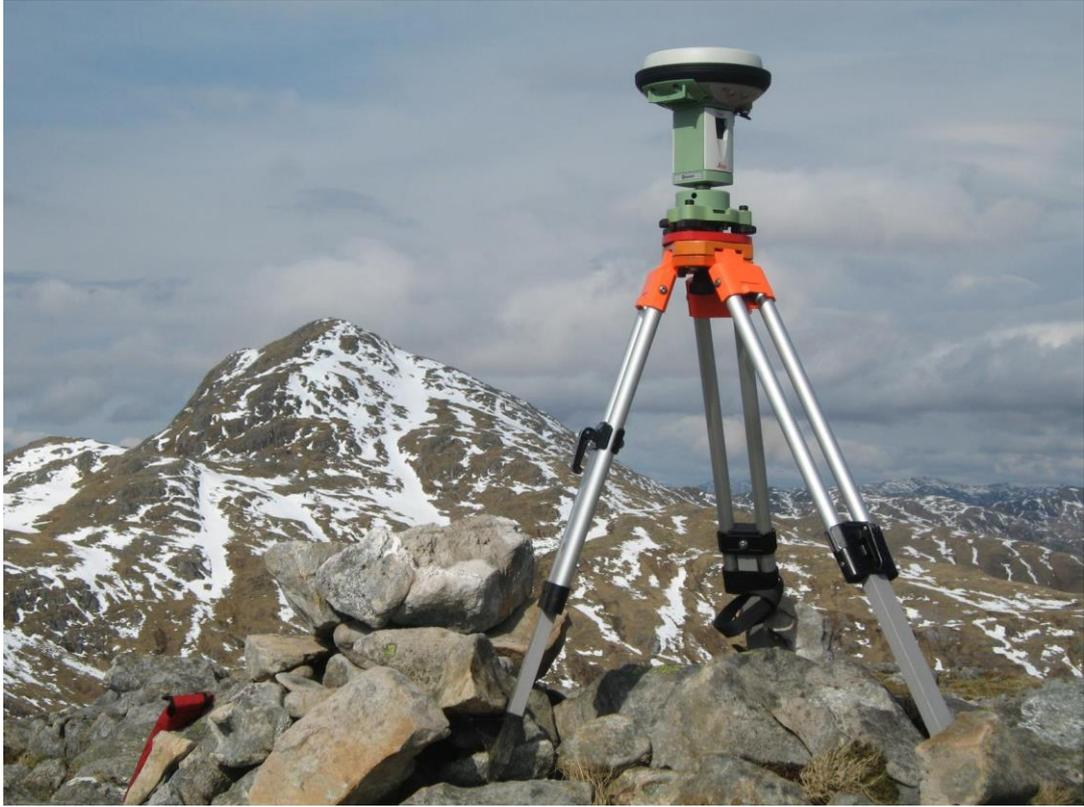
**Leica Viva GS15 collecting data at set-up position by cairn**
