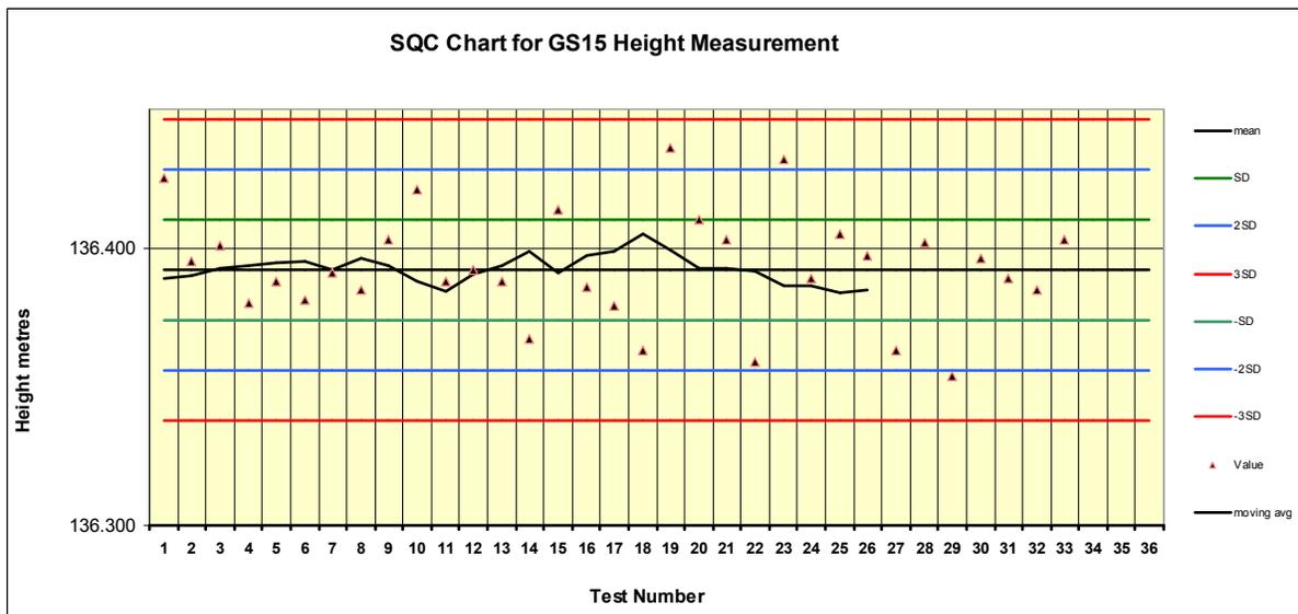
In addition, we check the instrument periodically by taking measurements on an Ordnance Survey Fundamental Bench Mark, processing the data and comparing it with the OS derived values. Height should agree within about 0.02-0.03m.
