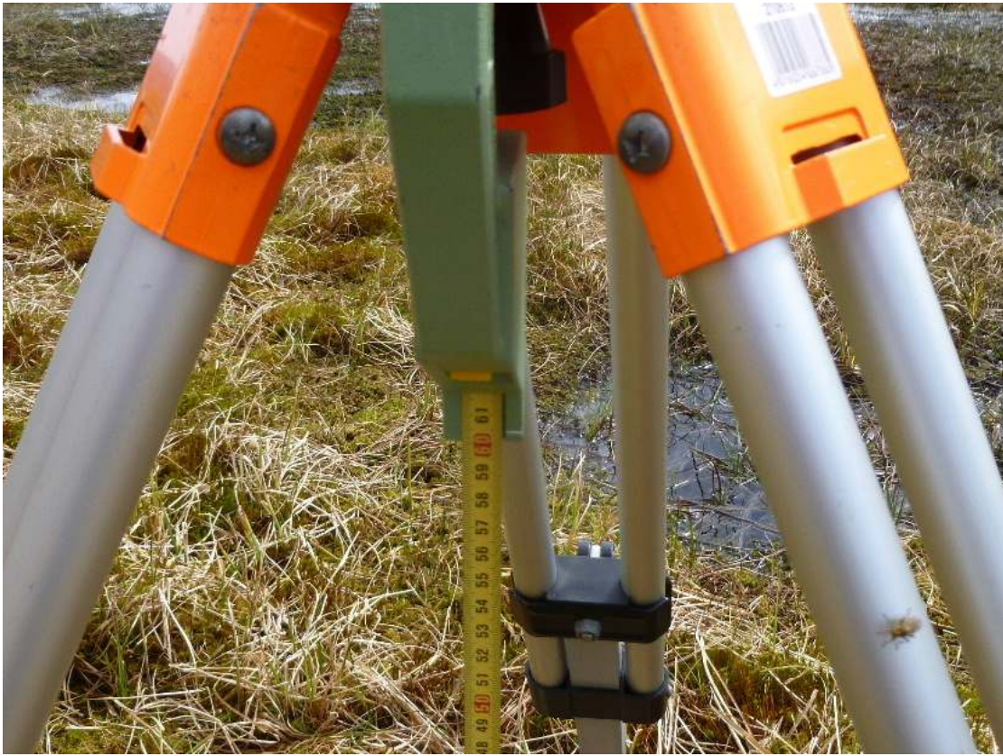
Measuring the Offset, 0.604m, for the GS15 on the beach
