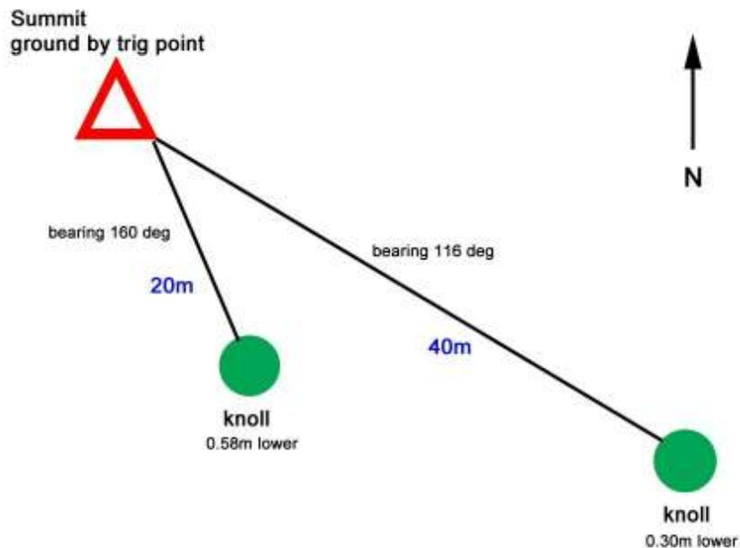
The Leica NA730 level was set up on a tripod at a convenient position and staff measurements were taken at possible summit candidates. The highest point was found to be ground adjacent to the trig point. The rocky knoll about 20m SSE of the trig point was measured to be 0.58m lower. The other main candidate about 40m ESE was measured to be 0.30m lower. Staff readings were also taken from the summit point and the Flush Bracket on the trig point.
