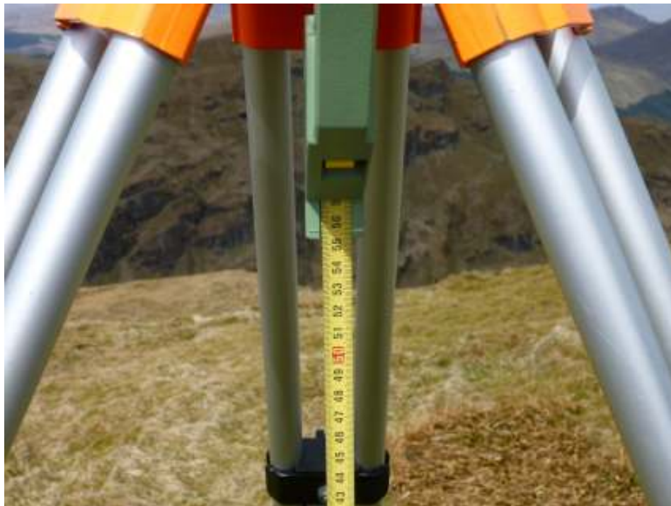
Measuring the offset, 0.556m, for the Leica Viva GS15 on the summit
