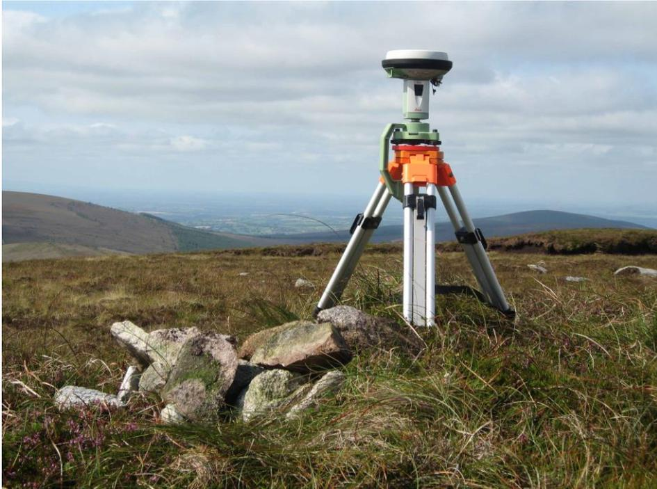
Figure 3: Leica Viva GS15 set up on summit
