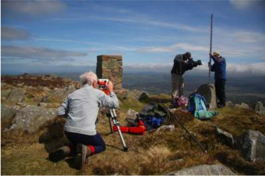
**Leica Viva\_GS15 set up on a 2.000m pole for summit measurement**
