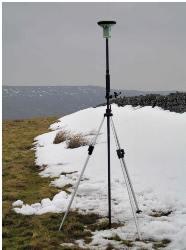
Leica GS15 set up on a 2metre pole over the summit of Thack Moor
