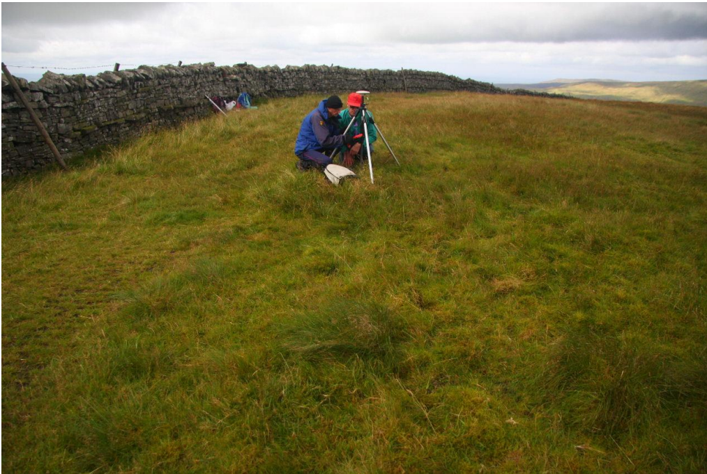
Leica SR530 set up on a 1 metre pole over the summit of Thack Moor
