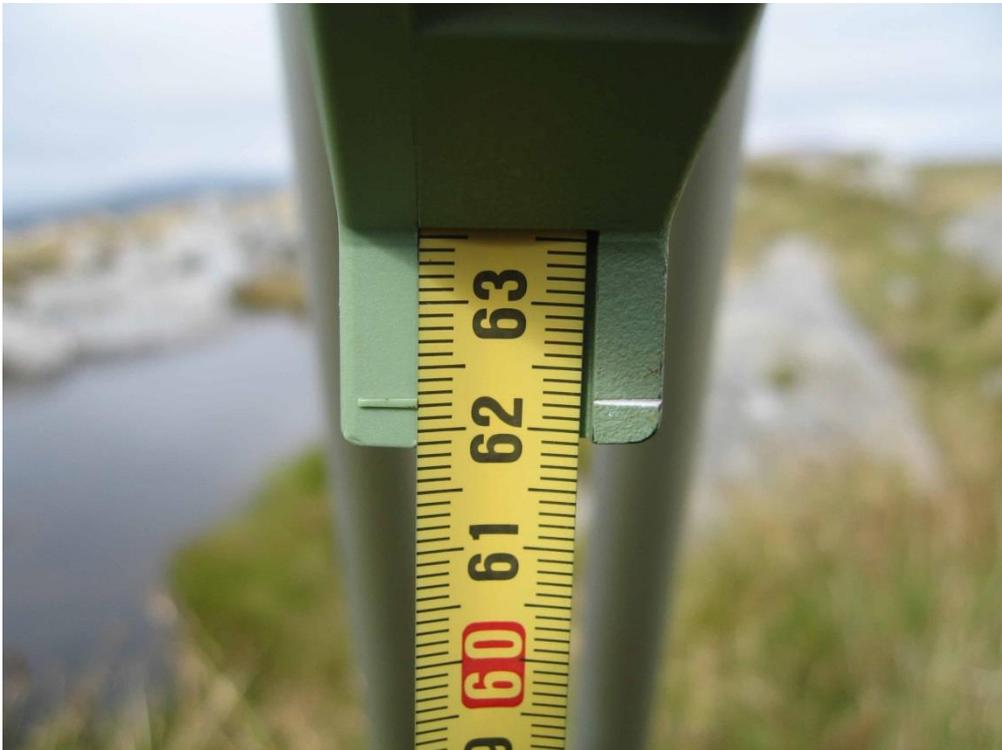
**Figure 4: Offset reading for Leica Viva GS15 set up at col of SW Top**
