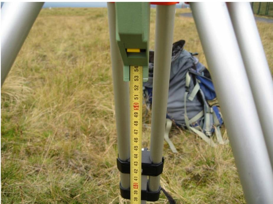
Figure 1: Offset reading for Leica Viva GS15 set up at reservoir summit position 2
