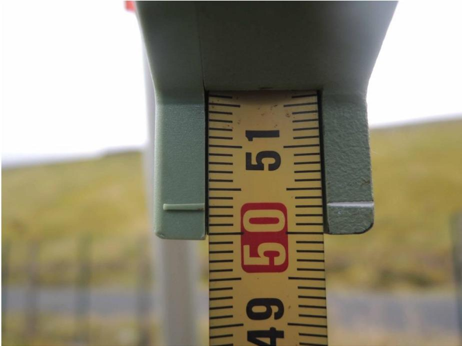
Figure 1: Offset reading for Leica Viva GS15 set up at reservoir summit position 1
