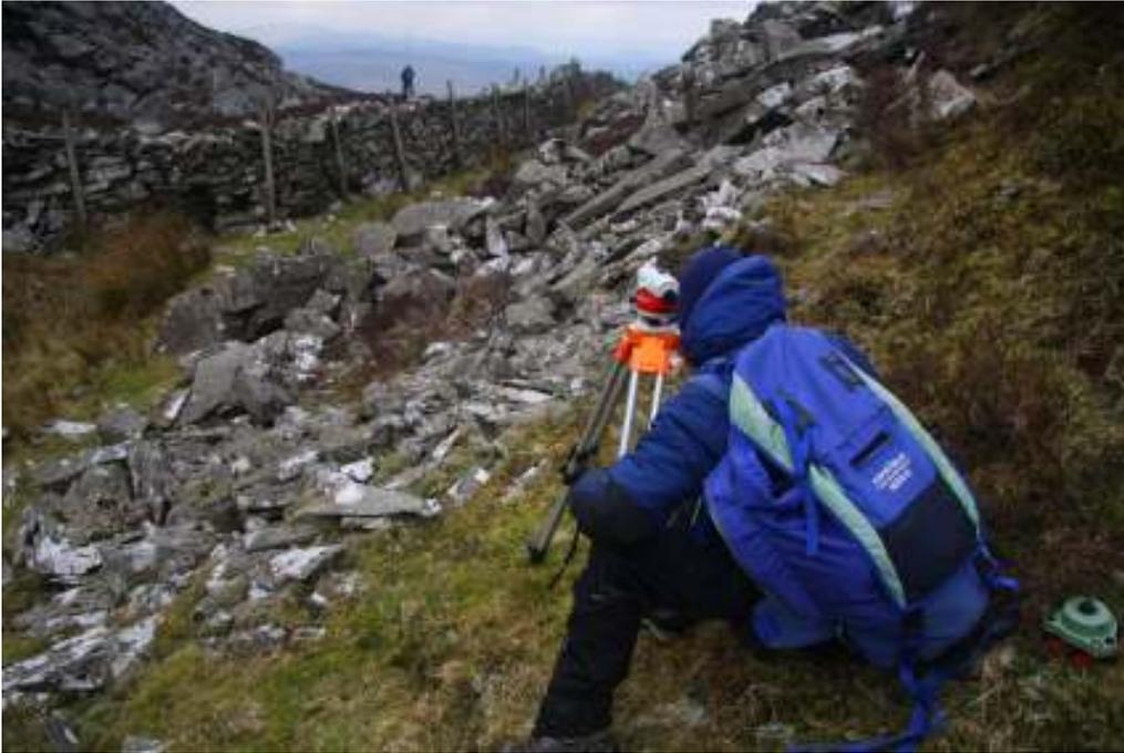
**Detail (0.502m) showing Tape Measurement from Ground level for Leica GS15 set up to measure bwlch height**
