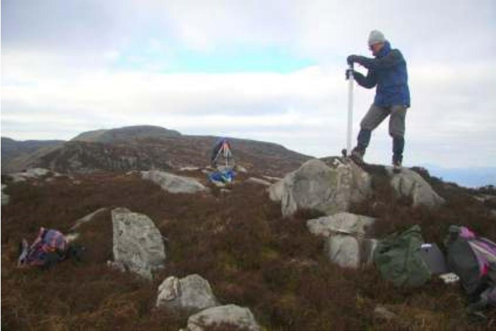
**Detail (0.601m) showing Tape Measurement from Ground level for Leica GS15 set up to measure summit height**
