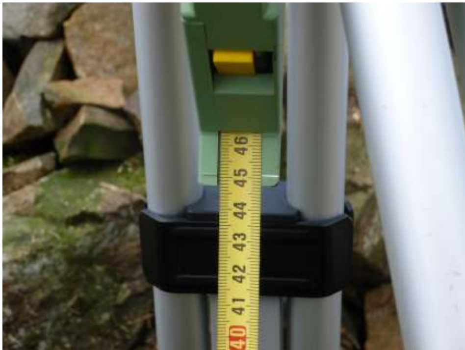
Measuring the offset for the Leica Viva GS15 on the summit of Cruachan Dearg
