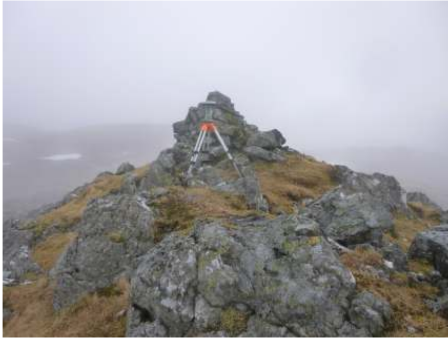
Leica Viva GS 15 collecting GNSS Data over Rock next to Summit Cairn
