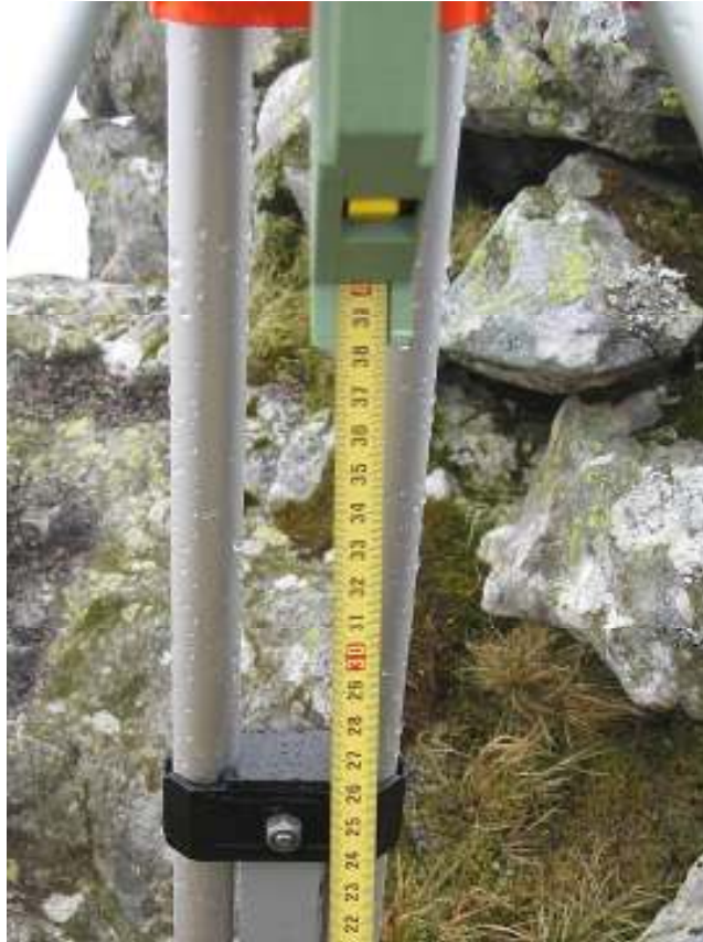
Measuring the offset for the Leica Viva GS15 on Beinn na h-Uamha
