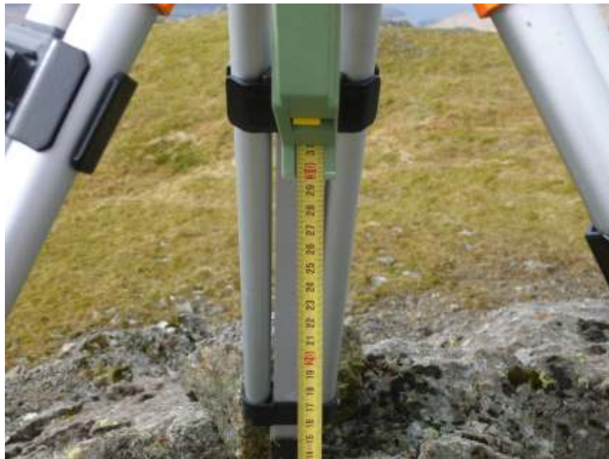
Measuring the offset for the Leica Viva GS15 on the summit of Corra-bheinn
