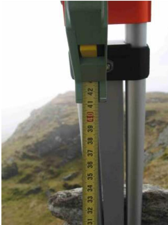
**Measuring the offset for the Leica Viva GS15 on Cnoc Coinnich**
