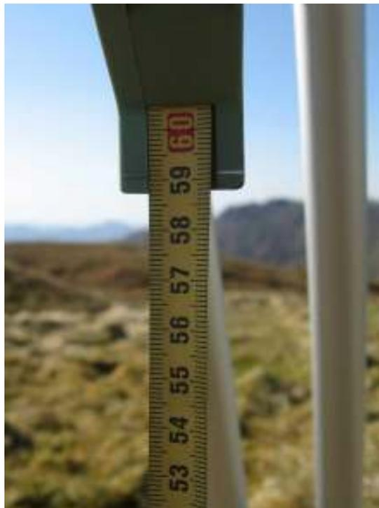
**Measuring the offset for the Leica Viva GS15 on Cruach nam Mult**
