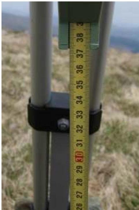
**Measuring the offset for the Leica Viva GS15 on Cruach nan Capull**
