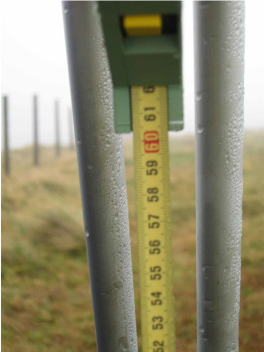
**Measuring the offset, 0.606m, for the Leica Viva GS15 on the summit of Uamh Bheag**
