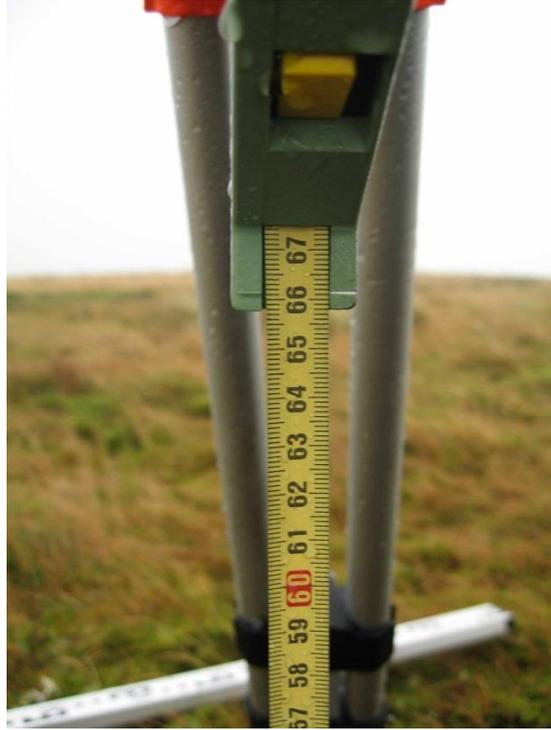
**Measuring the offset, 0.661m, for the Leica Viva GS15 on Uamh Bheag East Top**
