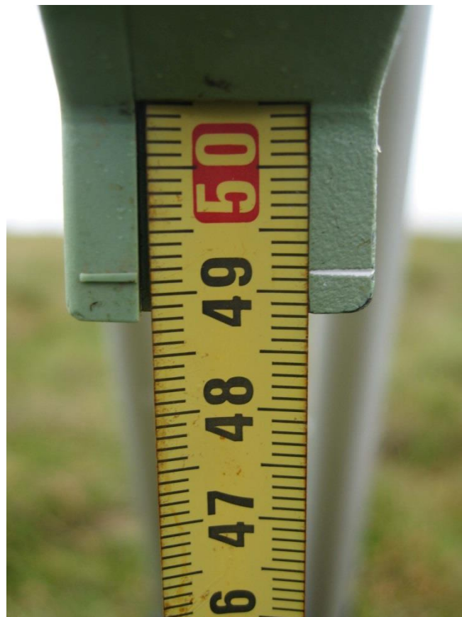
Tape reading for the Leica Viva GS15 on the summit
