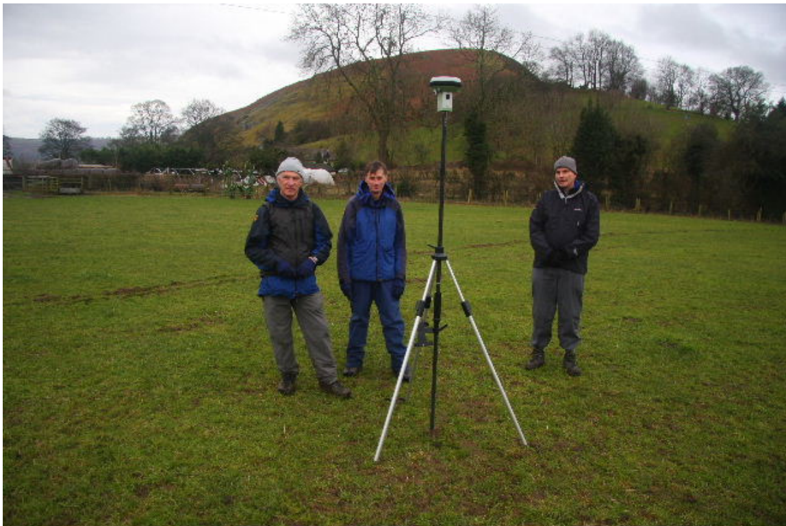
GPS set up for bwlch height measurement. (Bwlch behind row of trees)
