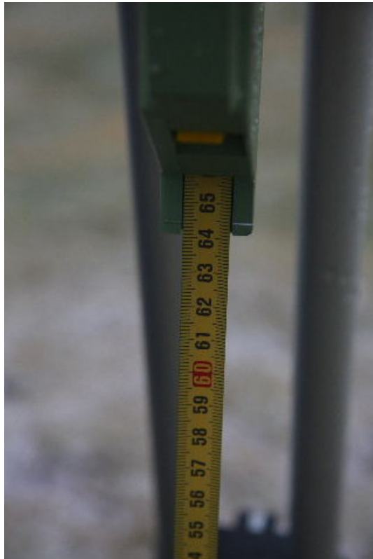
Leica GS15 set up showing vertical offset (0.644m) at the summit of Coed Hyrddyn
